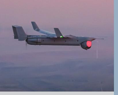
Integrator is designed to be a modular, flexible and multi-mission capable solution on land and at sea. With 50 pounds of payload capacity, the aircraft can be customized to support your operational needs. And because no nets or runways are required, your footprint stays small, even when your mission is not.
