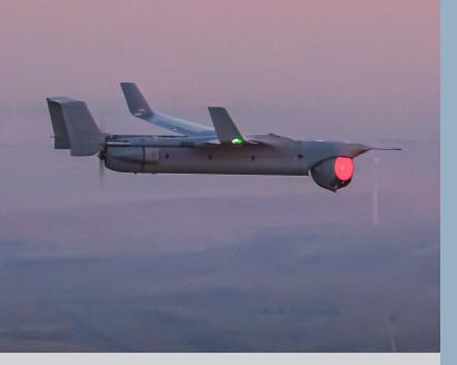
Integrator is designed to be a modular, flexible and multi-mission capable solution on land and at sea. With 40 pounds of payload capacity, the aircraft can be customized to support your operational needs. And because no nets or runways are required, your footprint stays small, even when your mission is not.
