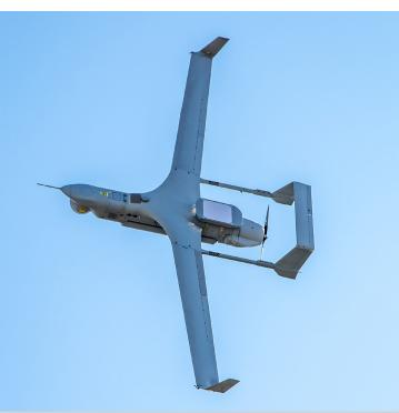
Integrator ER uses satellite communications (SatCom) to extend flight range beyond line of sight (BLOS), expanding target sets, reducing the logistical footprint and enhancing personnel safety.
